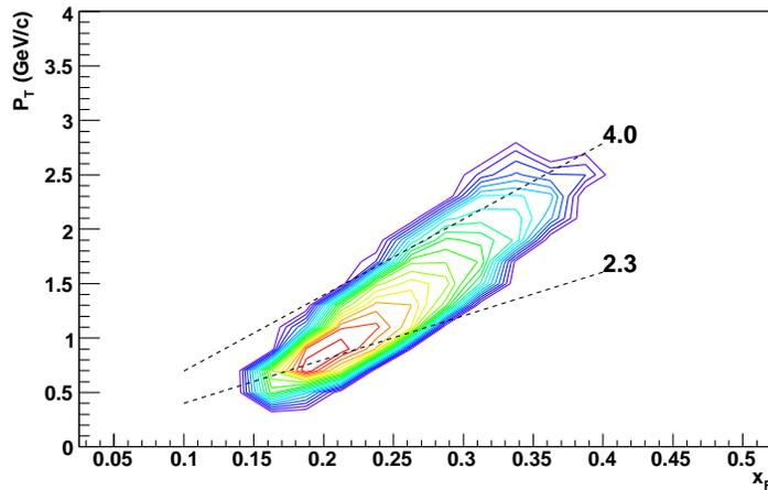
**FIGURE 1.** Acceptance in the BRAHMS experiment for pions at the nominal setting of 2.3 degrees in  $p_T$  vs.  $x_F$ . The dashed lines indicates the  $p_T$ -  $x_F$  correlations for fixed angles of  $2.3^\circ$  and  $4^\circ$ , respectively.
