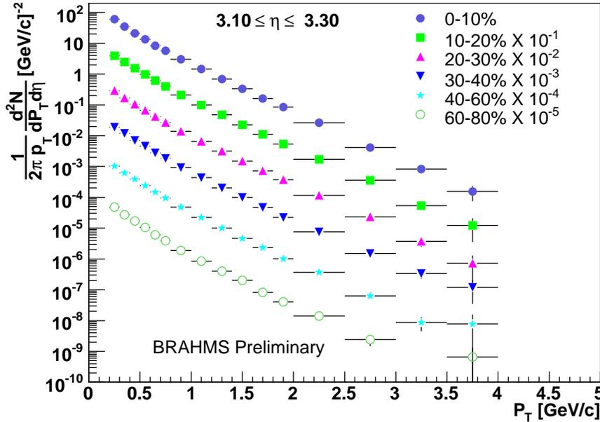
Fig. 1.  $p_T$  spectra at  $\eta$  3.2 in CuCu Collisions. The data are for six centrality bins and are scaled down for clarity by the indicated factors.
