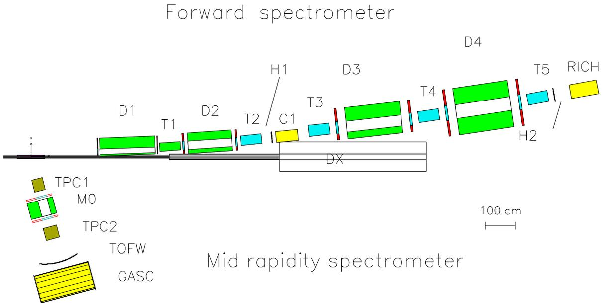
Figure 2. Layout of BRAHMS spectrometers. The names of individual components shown corresponds to the text where further details are given.
